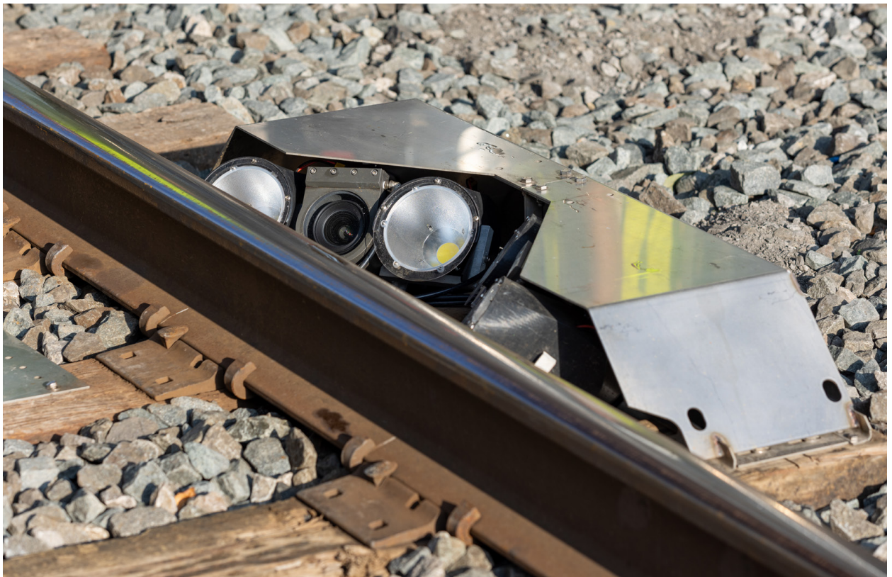
FIGURE 2. Cameras are installed strategically at various angles, including some at track level pointing up. (Courtesy of Norfolk Southern)
