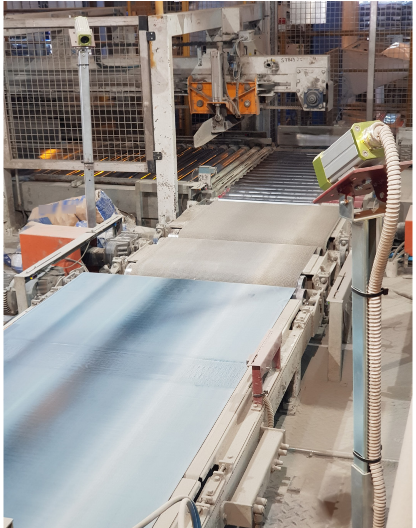
FIGURE 2. Two color cameras mounted above the production line inspect cement sacks for defects such as splits, cracks, and spills.
