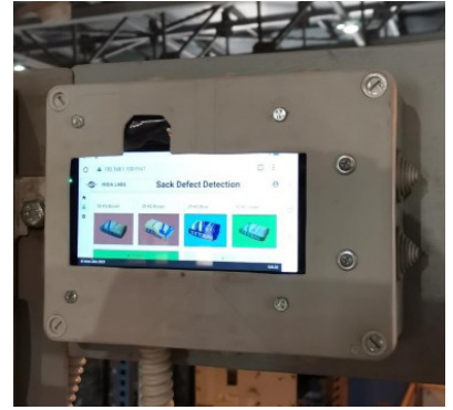
FIGURE 3. Image data from the cameras are transmitted to this edge computer, also mounted near the line, which identifies, analyzes, and takes necessary corrective action to remove defective bags from the line.
