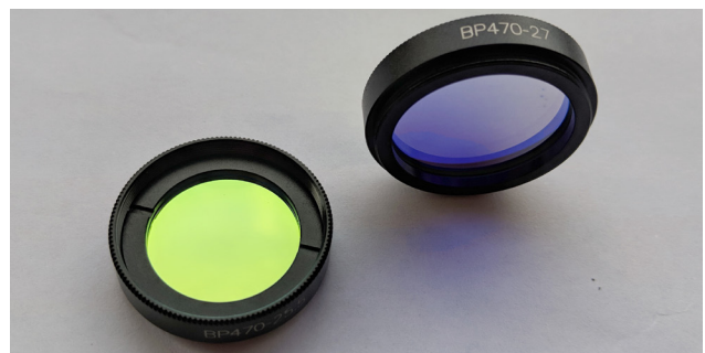
Figure 5: Two filters that only allow blue light to pass through are being used to show the difference between light being bounced back (reflection) and light passing through (transmission)
