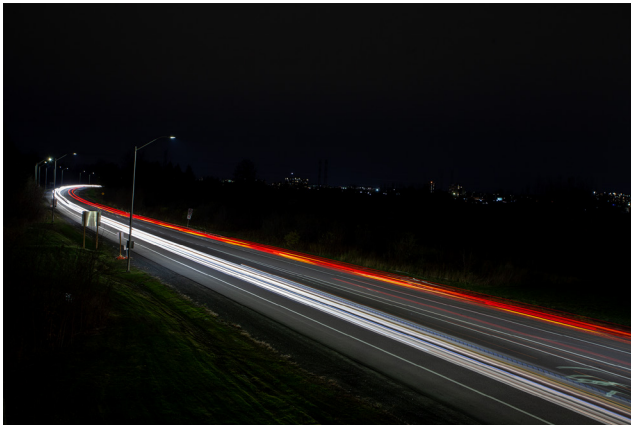
Figure 6: In traffic imaging a longer exposure can allow for more light to be captured but it will often lead to blurred vehicles, requiring a faster frame rate with additional lighting
