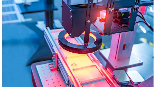
Figure 4: Ring lighting being used to inspect a metallic washer
