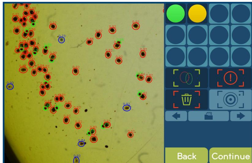
**FIGURE 1.** Using machine vision and AI, SnappArt automates the process of quantifying and assessing live feed used in hatcheries, such as the Rotifers pictured here. (*Courtesy of Aris BV*)
