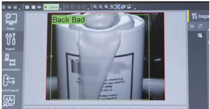
**FIGURE 4.** Federal Package trained the In-Sight 2800 from Cognex using images of deodorant containers in four categories: front good, front bad, back good, back bad. (Courtesy of Cognex Corporation)
