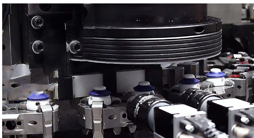
**FIGURE 1.** The inspection system checks bottle caps for cracks and flaws.
