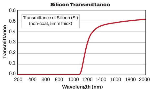
**FIGURE 2.** Transmittance plot for silicon that shows a high level of transmittance for wavelengths over 1100 nm.
