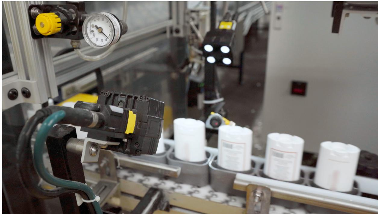
**FIGURE 1.** Vision system classifies cosmetic defects on deodorant containers. (Courtesy of Cognex Corporation)
