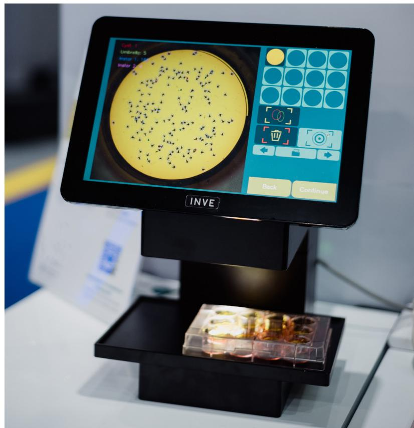
**FIGURE 2:** SnappArt can count a sample in less than one minute and then results are available immediately. (*Courtesy of Aris BV*)
