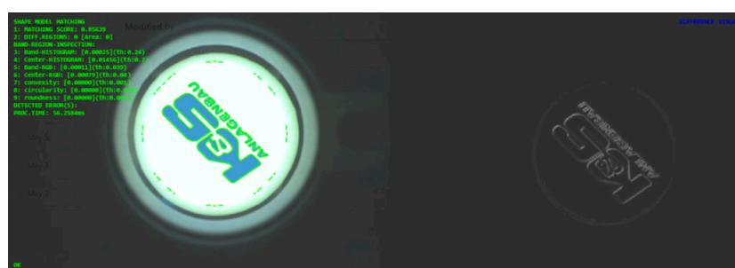
**FIGURE 4.** The GUI showing that the imprint on the top of the bottle cap is “OK.”
