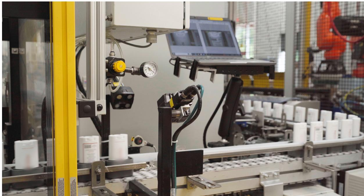
**FIGURE 3.** To inspect deodorant containers, Federal Package set up two cameras, with each one taking a picture of one side of a deodorant container as it moves through the line. (*Courtesy of Cognex Corporation*)
