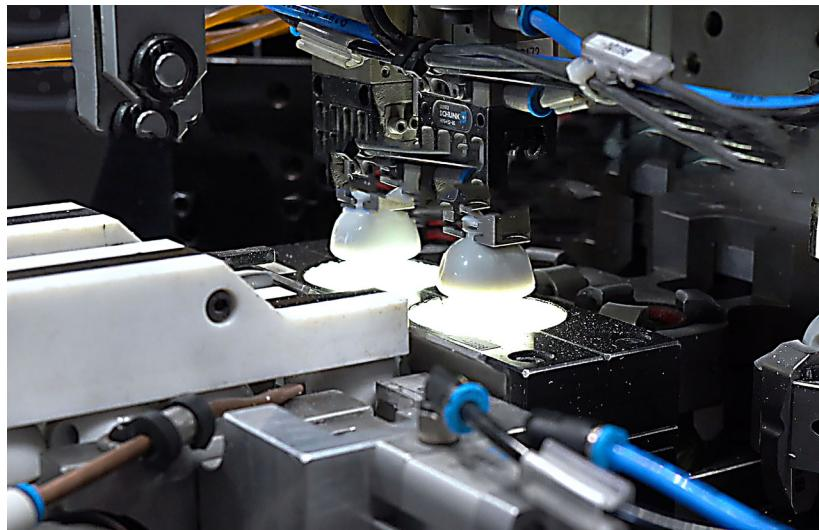
**FIGURE 2.** The system inspects the bottle cap tops for print and image errors.
