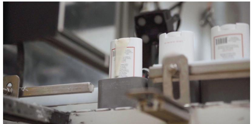
**FIGURE 2.** Federal Package developed an automated process to spot drips and other imperfections on deodorant containers. (Courtesy of Cognex Corporation)
