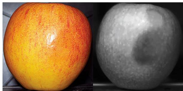
**FIGURE 3.** SWIR imaging is great for moisture identification because of water's SWIR absorption, which is useful in fruit inspection. This makes moisture visible that would be otherwise very difficult to identify.
