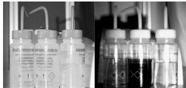
**FIGURE 4.** Isopropanol, water, and acetone look essentially identical under visible light, but SWIR imaging results in high contrast between them, making it easy to differentiate between them.
