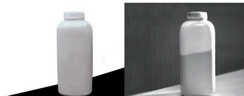
**FIGURE 1.** SWIR cameras and lenses can look through some objects that are opaque under visible light, like this white bottle, to reveal the hidden substances inside them. (Photos & images/Edmund Optics)
