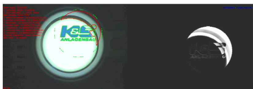
**FIGURE 3.** The GUI shows that the imprint on the bottle cap is “not ok.”
