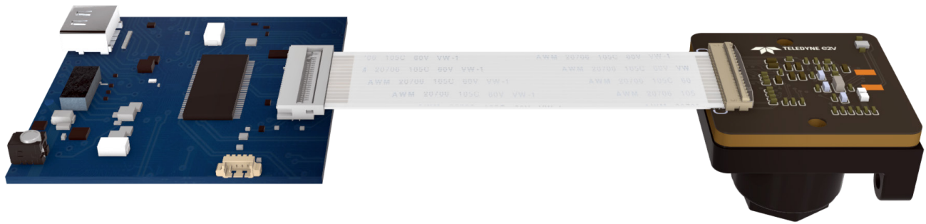
FIGURE 2. New modules (on the right) allow direct connection to off-the-shelf processing boards (on the left) through flat cables without the need to design any additional boards.
