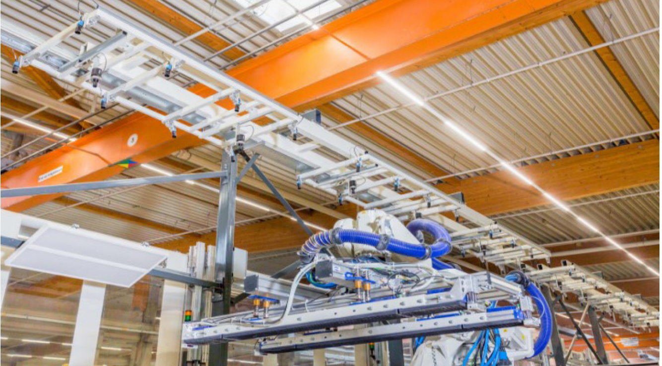
FIGURE 3: A robotic cell and vision system coordinates the placement and positioning of sheets used in wall fabrication.
