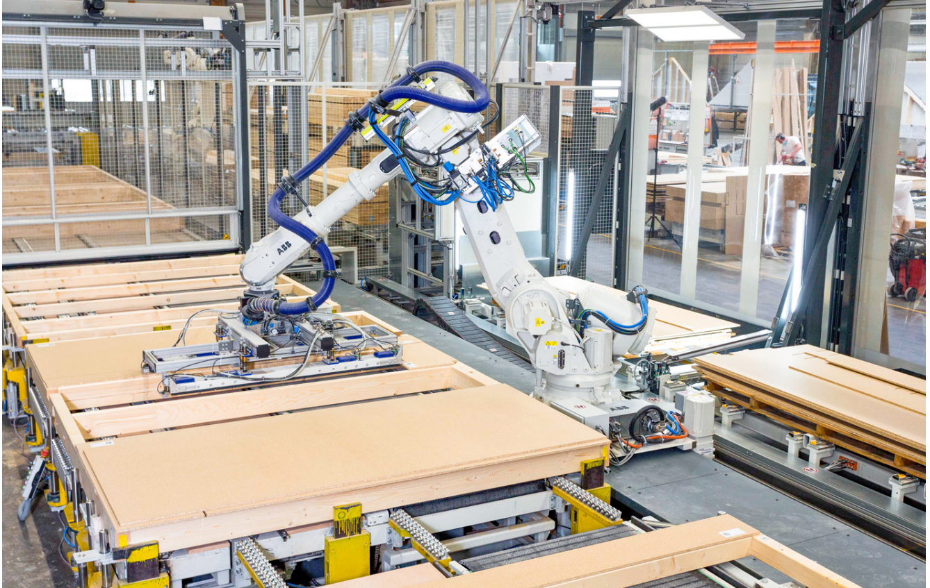
FIGURE 1: A robotic cell with a gripper system was used in combination with a 3D camera.
