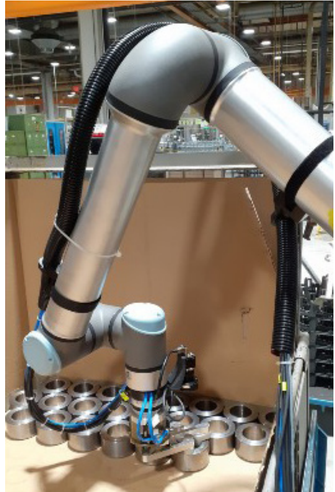
FIGURE 3: This photo shows an application with ZF, a global technology company headquartered in Friedrichshafen, Germany. It uses the Micropsi MIRAI robot control system to automate machine tending in a high-volume milling station where gears are manufactured.
