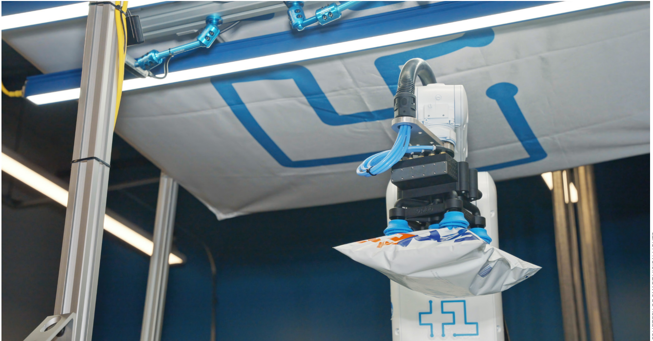
FIGURE 3: The robotic system from Plus One Robotics typically includes a lighting source, 3D camera, robotic arm, and industrial PC. (Picture does not show actual installation at a customer's site.)
