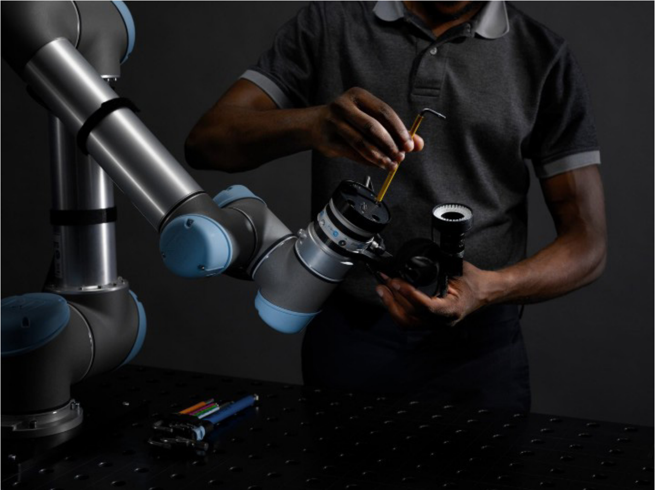
FIGURE 2: To get started with the MIRAI system, designers simply connect the robot, the F/T sensor, the camera(s), and the MIRAI controller. Set up time typically takes 30-45 minutes.
