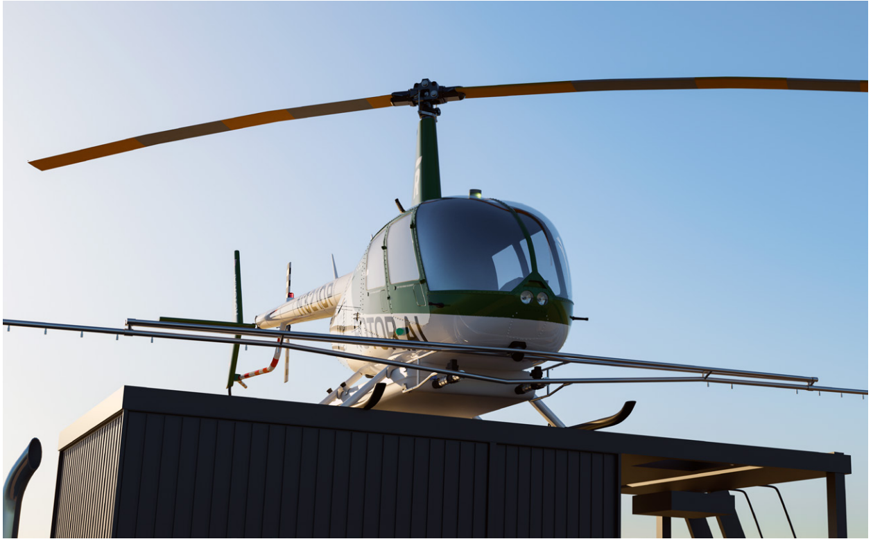
FIGURE 2. A Sprayhawk can land and take off from small platforms, such as the top of a truck used to transport it to the area where it will perform its mission.
