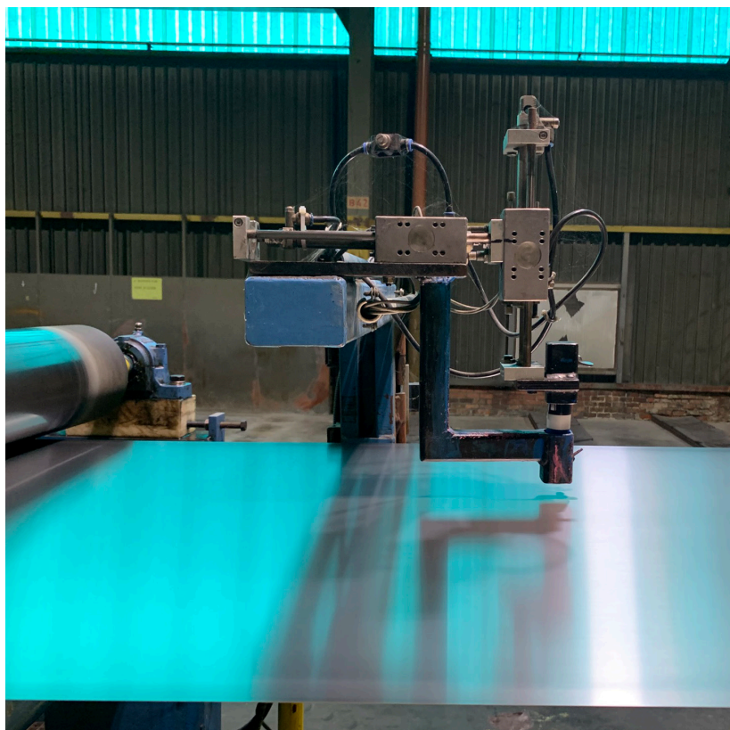
FIGURE 1. The integrators chose a contact image sensor because it acquires high-resolution images at high frequency.
