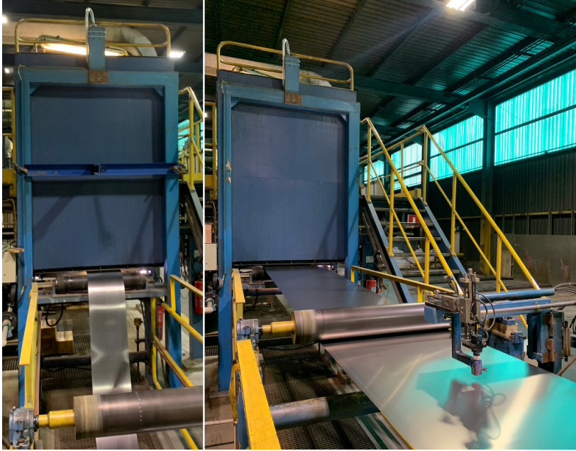
FIGURE 2. At TI Fluid Systems, steel strips move on a production line at a rate of 95 meters per minute, or 1,580 mm per second.
