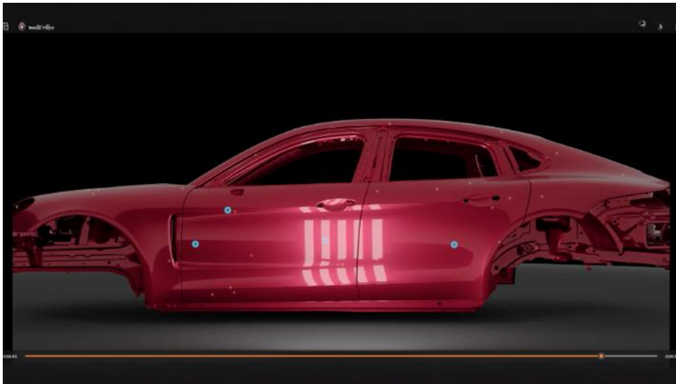
Figure 2 This image from Porsche (Stuttgart, Germany) illustrates how a known pattern of light is distorted by specific features when it is projected on an object.
