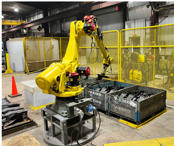
FIGURE 3. Penna Flame Industries purchased a FANUC R 2000/165F robot to automate the process of packaging leaf spring support arms. Courtesy of Catalyst Connection
