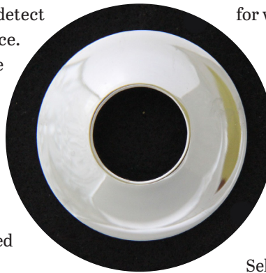
FIGURE 3. Part with a shiny (specular) finish. Courtesy of Perry West, Automated Vision Systems
