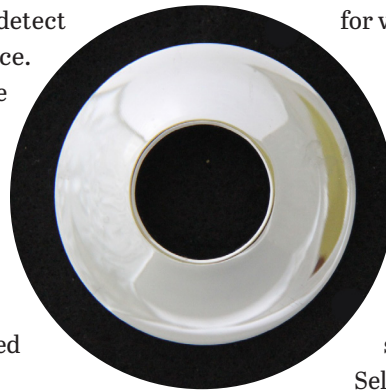
FIGURE 3. Part with a shiny (specular) finish. Courtesy of Perry West, Automated Vision Systems
