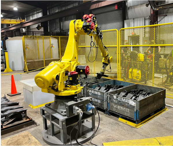
FIGURE 3. Penna Flame Industries purchased a FANUC R 2000/165F robot to automate the process of packaging leaf spring support arms. Courtesy of Catalyst Connection
