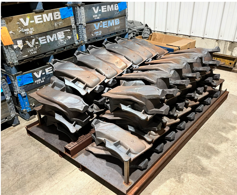
FIGURE 1. A steel component in vehicle suspension systems, each leaf spring support arm weighs 37 pounds, has dimensions of 18 × 12 in. and semi-sharp edges, and is irregularly shaped. Courtesy of Catalyst Connection
