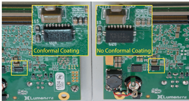
Figure 4. Comparing two identical circuit boards - one with conformal coating, one without
